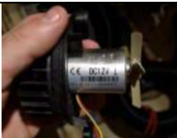
EXX-001-390 Combustion Fan Assembly
