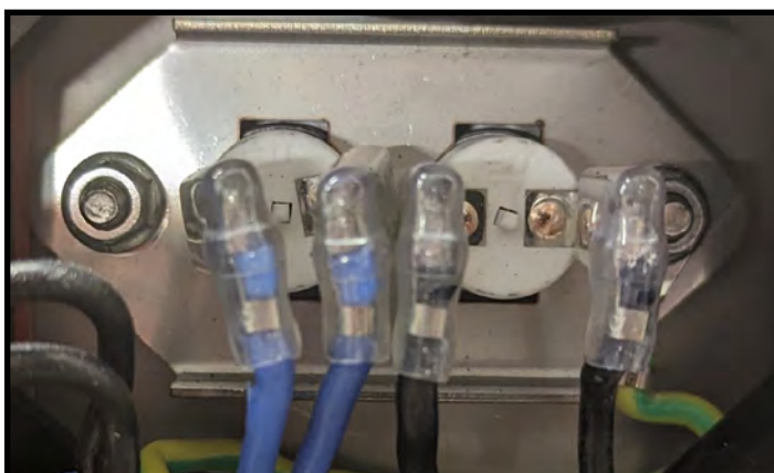
ELX-001-380 Water Tank Temperature Overheat Trigger (Updated Diesel/Gasoline Version)
