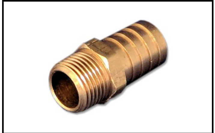
PLX-A65-200 Fitting, Brass Barb, 3/4" x 1/2" (M) NPT
