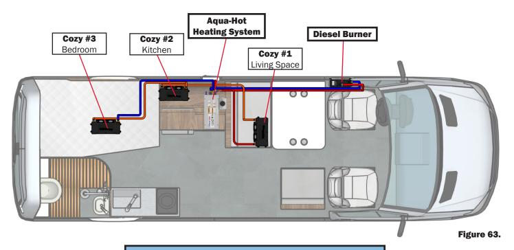
**NOTE:** This is just a sample for the layout of the diesel burner with the Aqua-Hot and heat exchangers. Actual placement may vary on the individual design of the RV. For questions or assistance, contact Aqua-Hot at 574-AIR-XCEL (574-247-9235).
