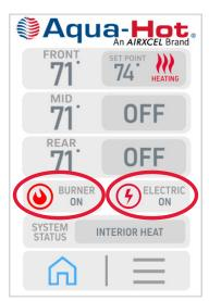
For continuous hot water or heat in colder conditions, it is recommended to utilize the external diesel burner. The electric heating element will provide heat only in mild conditions and provide light duty hot water needs.
