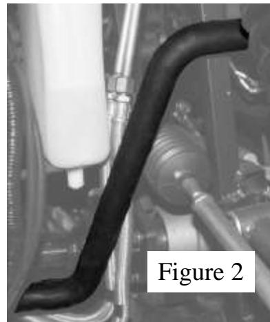
Make sure there is room for two,  $\frac{3}{4}$ " heater hoses to run from the Heater location to the Diverter Manifold.
