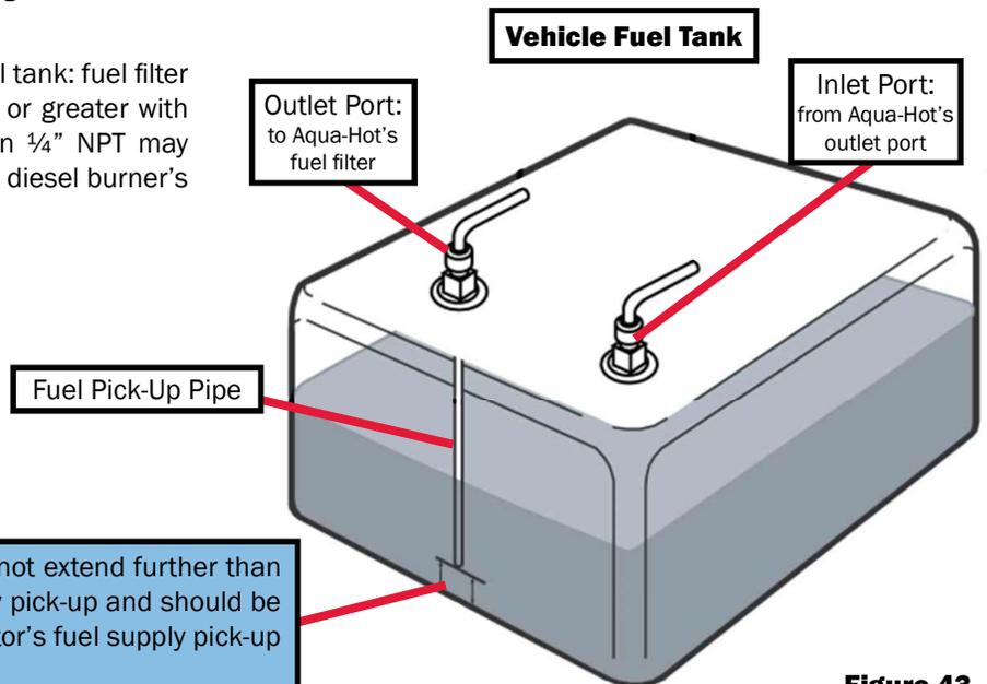
**NOTE:** The fuel pick-up pipe should not extend further than the motor home's engine fuel supply pick-up and should be consistent with the on-board generator's fuel supply pick-up length.
