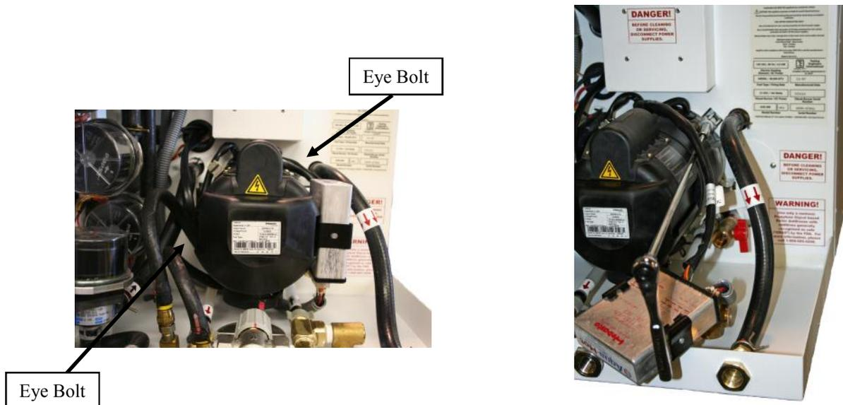
1. The Diesel-Burner is secured to the Aqua-Hot with two Eye Bolt Nuts that can be loosened, and swung out of the way by using a 10mm socket wrench with a 10 inch long extension.
