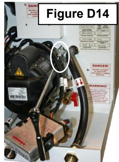
1. Align the Diesel-Burner with the Hydro-Hot, using the alignment tabs welded on the Hydro-Hot.
