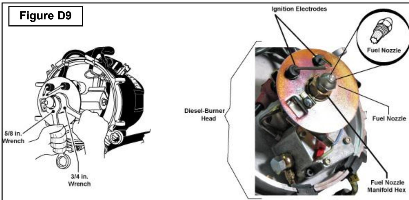
**NOTE:** It is recommended to check fuel pressure any time the fuel nozzle is replace.
