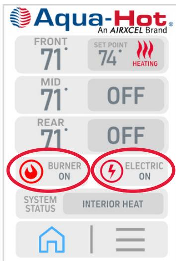
For continuous hot water or heat in colder conditions, it is recommended to utilize the external diesel burner. The electric heating element will provide heat only in mild conditions and provide light duty hot water needs.
